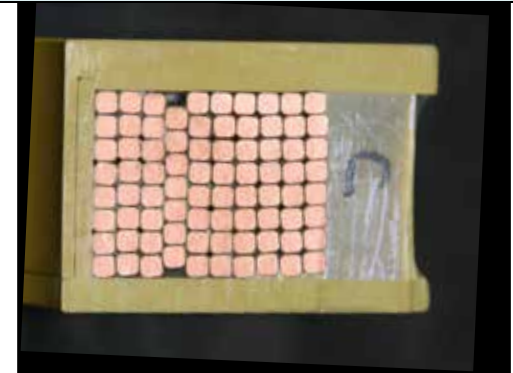
Cross section of coil showing Cu wire, Torlon housing, and Zylon/epoxy reinforcement
